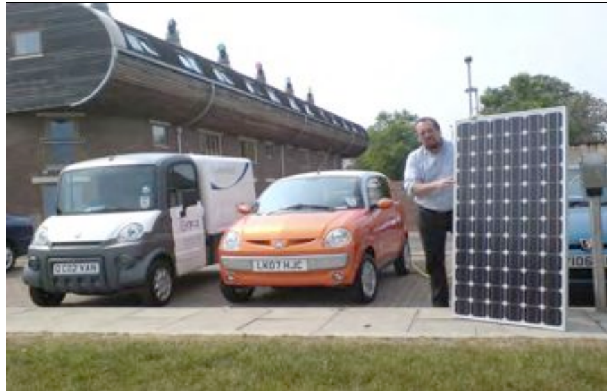
This 190 watt pv panel could approximately power an electric trike for around 1000 miles/ year in the uk and an electric car half this distance – making zero carbon personal transport possible in suburban and rural areas with low PTAL ratings.
